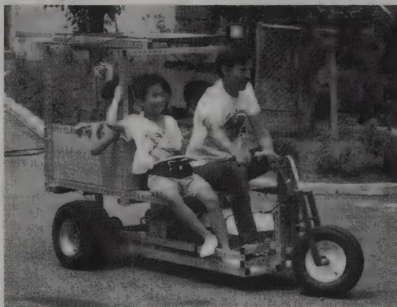
This solar vehicle was built in California in 1991 for a solar-energy workshop at a school in Japan. For the trip, the machine was taken apart and rebuilt as its own packing containers with travel clothes padding the components. The three containers went on the airplane as luggage. The vehicle was then re-assembled in Japan by children. I'll bet they remember it a long time.
